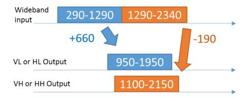
The diagram above shows the basic frequency relation between wideband satellite frequencies and the standard legacy satellite frequencies. Below is the relation between the STB tuned transponder and the wideband incoming transponder frequency.
